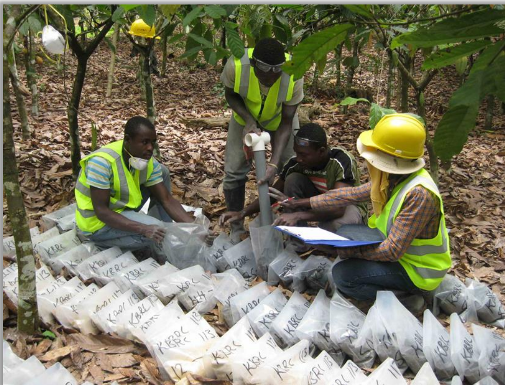
Figure 10.5 Reserve Circulation Sampling Using Tube Splitter
