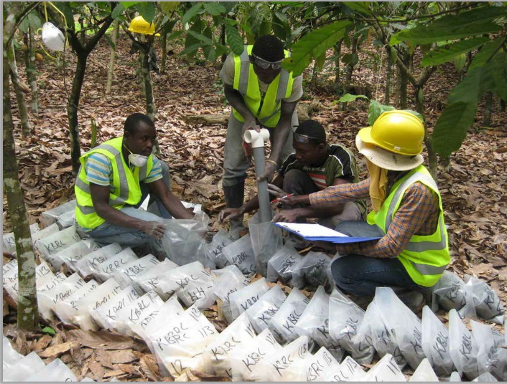
Figure 10-5 - Reserve Circulation Sampling Using Tube Splitter
