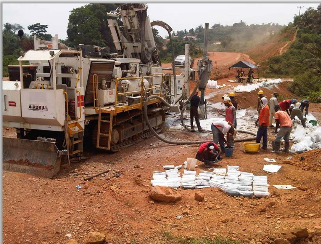
Figure 10-2 - Reserve Circulation Drill
