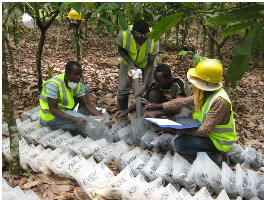
Figure 10.5 Reserve Circulation Sampling Using Tube Splitter
