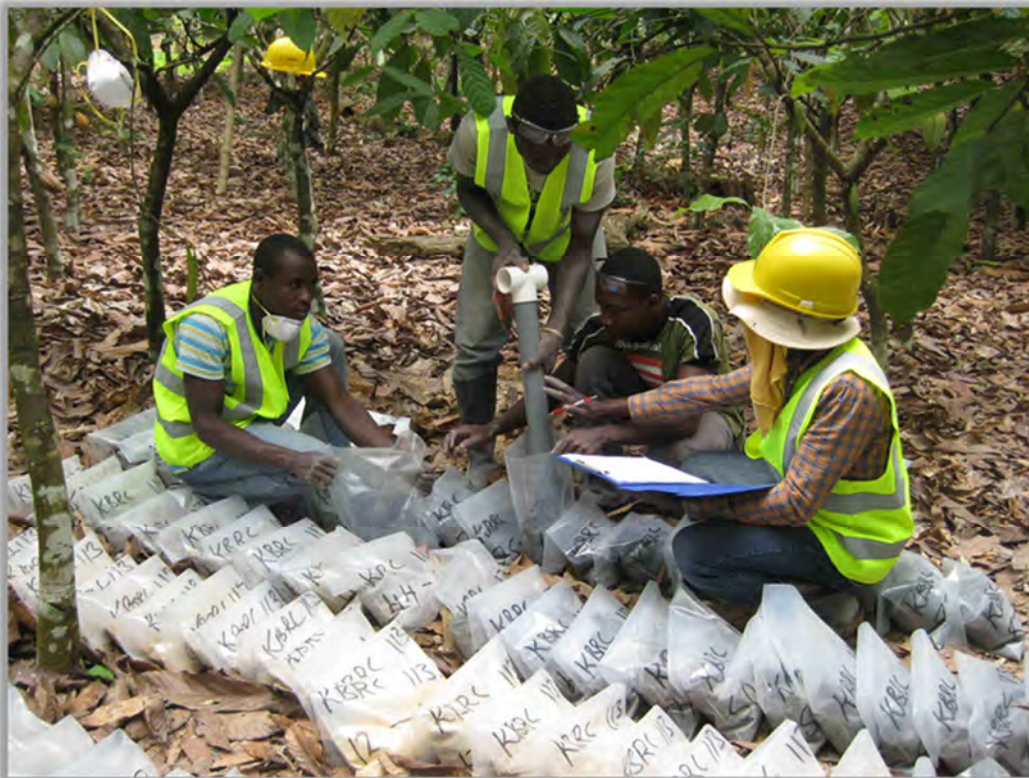
Figure 10.14 Reverse Circulation Sampling Using Tube Splitter
