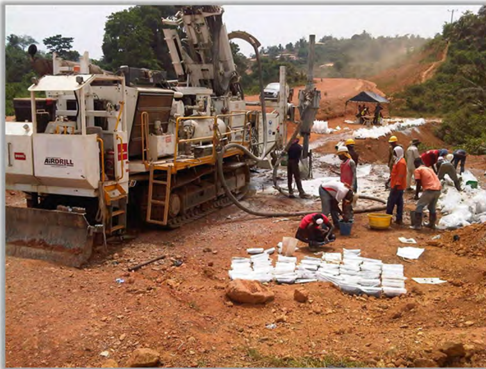
Figure 10.8 Reverse Circulation Drill
