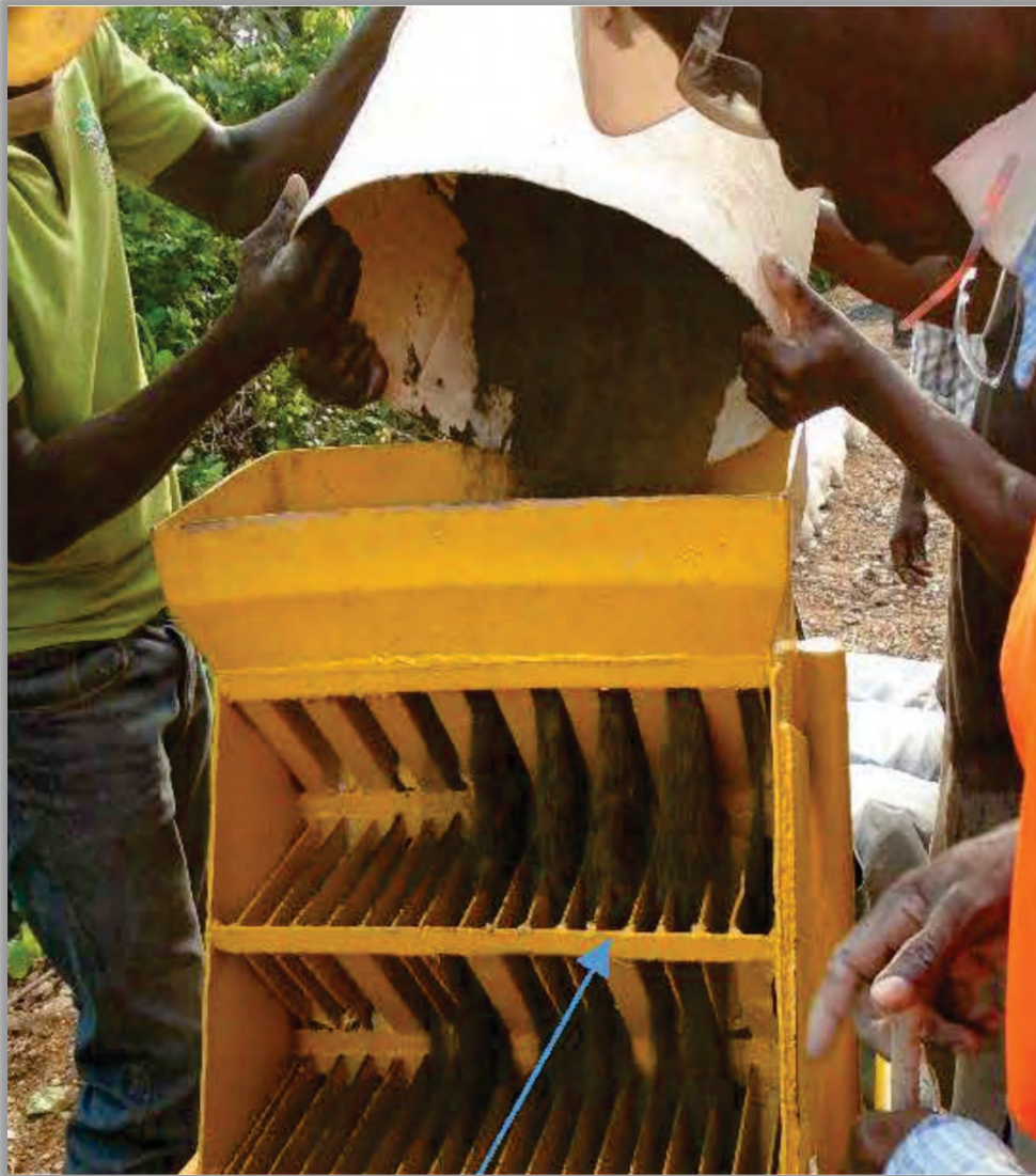
Figure 10.15 Reverse Circulation Sampling Riffle Splitter
