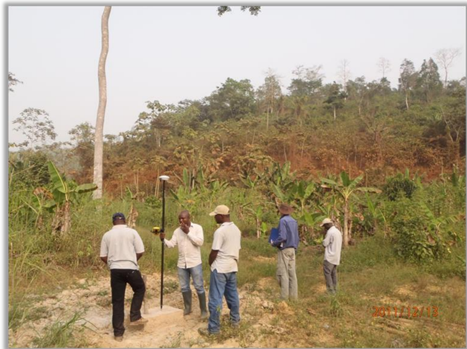
Figure 10-13: Collar Survey (McCracken, 2012)
