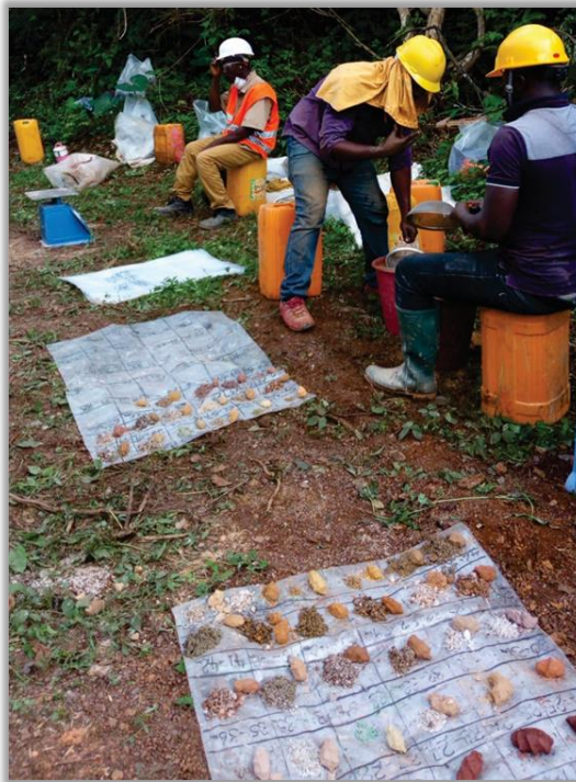
Figure 10-15: RC Chip Logging (Newcore, 2017)
