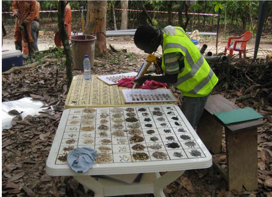
Figure 10-16: Chip Board Preparation (Newcore, 2017)
