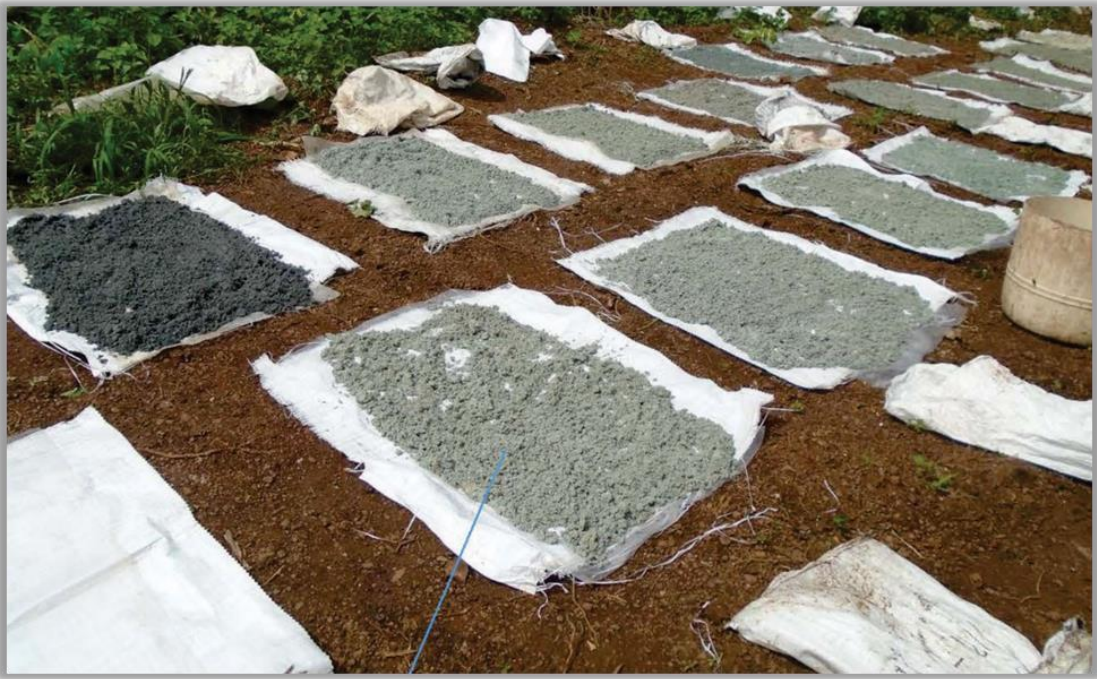
Figure 10-19: Drying Wet RC Samples (Newcore, 2017)
