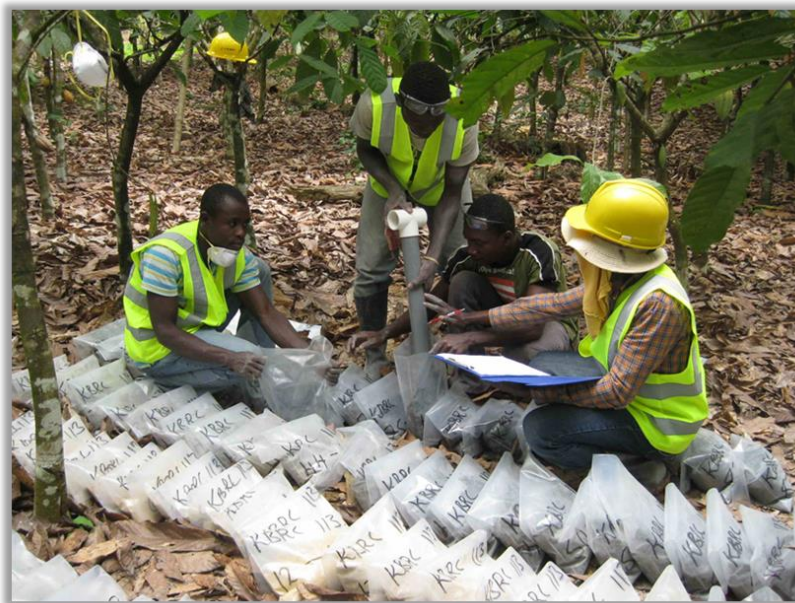
Figure 10-17: Reverse Circulation Sampling Using Tube Splitter (Newcore, 2012)
