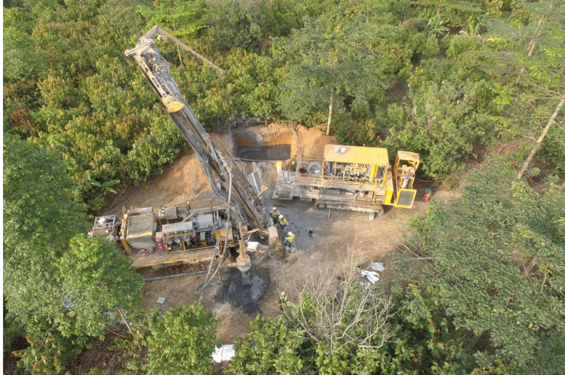
Figure 10-14: Reverse Circulation Drill (Newcore, 2021)
