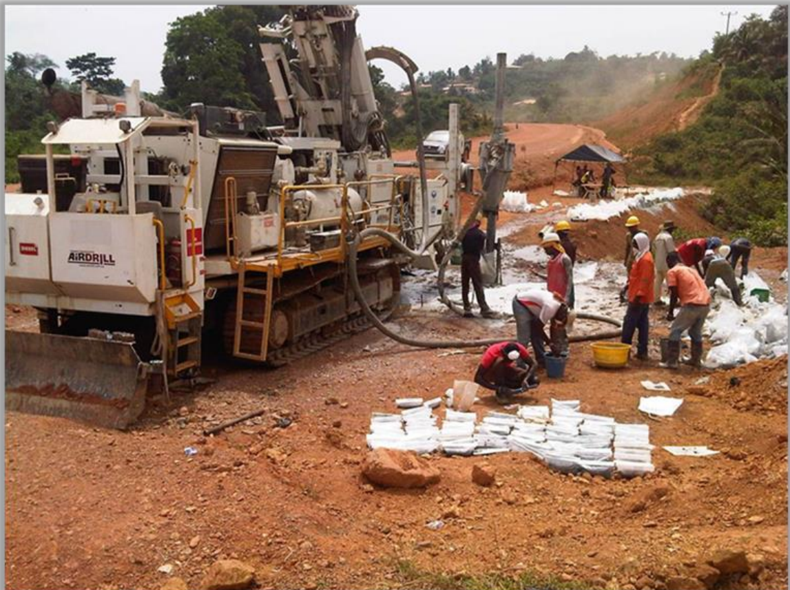
Figure 10-5: Reverse Circulation Drill (Newcore, 2012)
