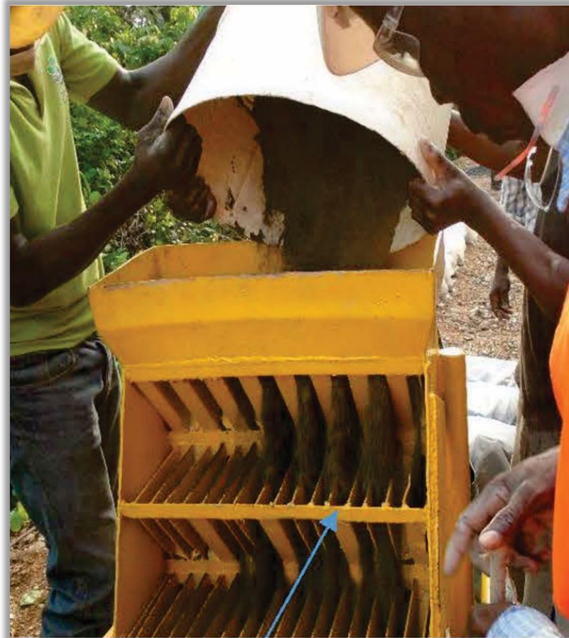
Figure 10-18: Reverse Circulation Sampling Riffle Splitter (Newcore, 2017)
