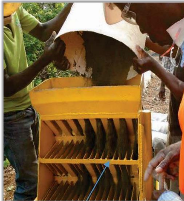
Figure 10.13 – Reverse Circulation Sampling Riffle Splitter
